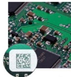
Machine vision provides the high-speed alignment and traceability for electronics assembly, even on the newest miniaturized components and flexible circuits.
