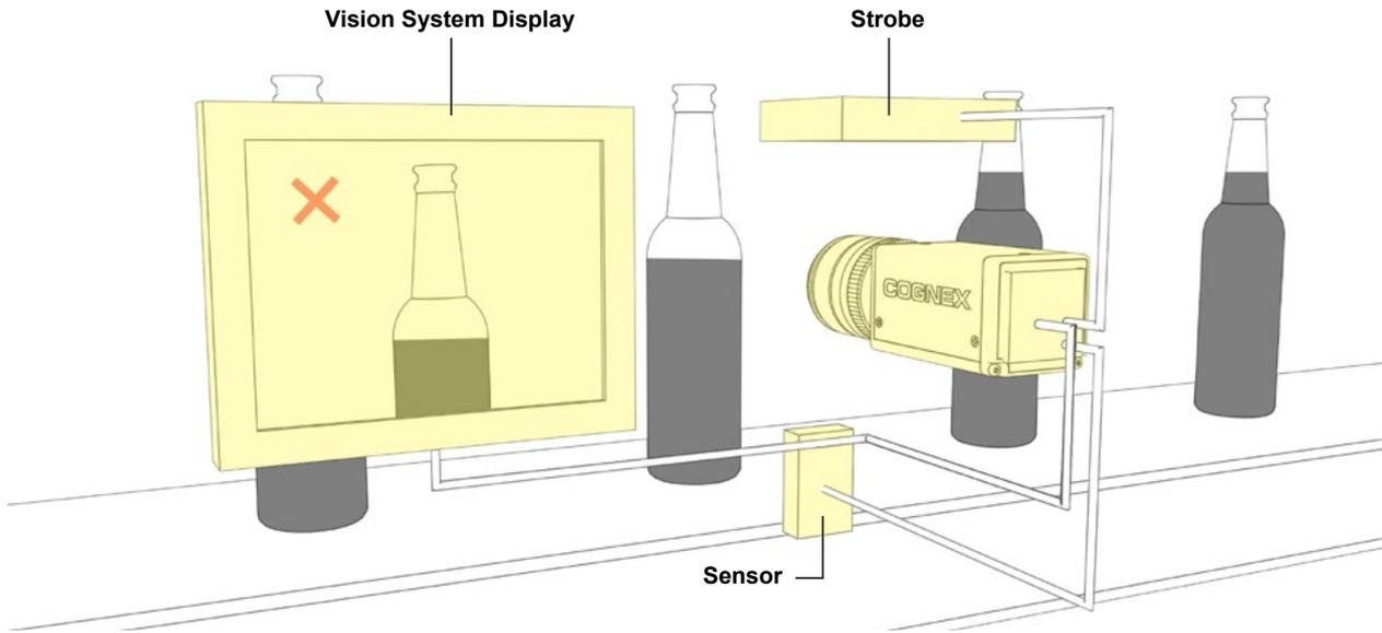
**Figure 1.** Bottle fill-level inspection example
