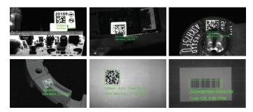
1DMax with Hotbars technology deliver high-speed reading of damaged or poorly printed 1-D barcodes as small as 0.8 pixels per module (ppm).
