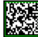
Quiet zone violation
