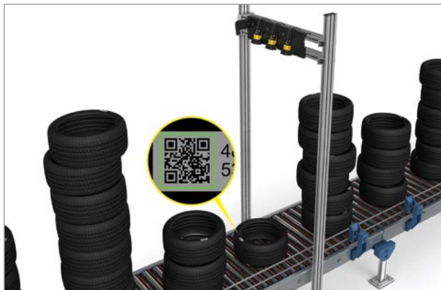
Image-based barcode readers with high speed liquid lenses rapidly read codes at different heights on tires, regardless of orientation.
