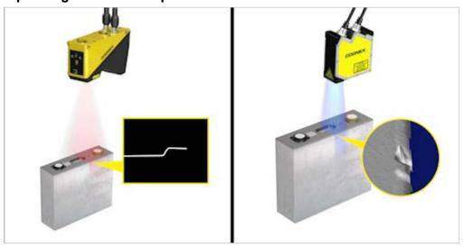
The DS1000 3D laser displacement sensor measures the height difference between the cap and battery case prior to welding. Afterwards, the DS925 laser displacement sensor inspects the welded seams to ensure they are fully sealed and free of defects.
