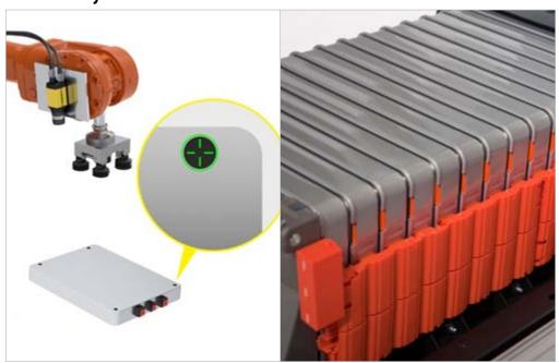
The In-Sight 8000 vision system guides the final assembly of modules and cable connectors into a pack.
