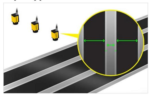
Cognex Industrial Area Scan Cameras and VisionPro software gauge the dimensions of the separator and electrode.
