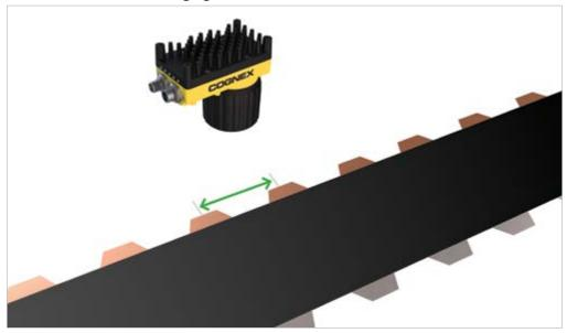
The In-Sight® 5000 vision system measures the distance between poles on a cell sheet.
