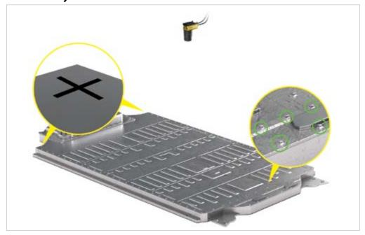
The In-Sight 9912 vision system inspects the final battery pack for completeness and fixtures it for robotic placement.
