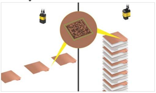
DataMan® image-based barcode readers read laseretched DataMatrix codes on the copper sides of cell sheets and the top of stacked electrodes.
