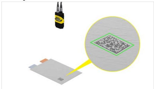
A DataMan 260 imagebased barcode reader reads stretched DataMatrix codes on a pouch's surface.
