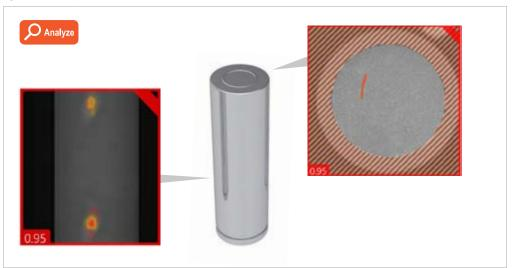
Cognex ViDi™ deep learning-based image analysis software inspects a cylinder battery for surface defects.
