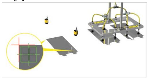
Cognex Industrial Cameras and VisionPro software align cell sheets for stacking.
