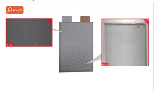
Cognex ViDi deep learning-based software identifies surface defects, like bubbles and wrinkles, on a pouch's surface.
