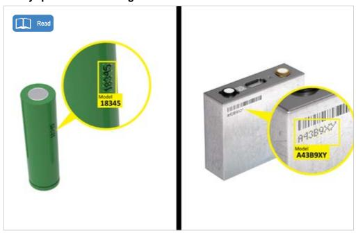
Cognex ViDi locates and reads the alphanumeric codes on batteries using a pre-trained font library.
