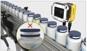
3D laser displacement sensors optimize product quality by providing accurate, micron-level 3D inspection. A laser displacement sensor placed above open boxes uses 3D measurements to ensure that the cap on every bottle inside is properly positioned. Mis-assembled caps are flagged before the box is closed and placed on a truck for delivery. This helps avoid spills and quarantines defective product before it leaves the facility.
