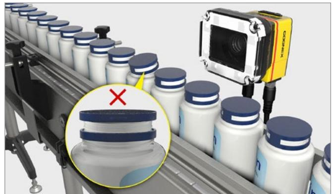
3D laser displacement sensors optimize product quality by providing accurate, micron-level 3D inspection. A laser displacement sensor placed above open boxes uses 3D measurements to ensure that the cap on every bottle inside is properly positioned. Mis-assembled caps are flagged before the box is closed and placed on a truck for delivery. This helps avoid spills and quarantines defective product before it leaves the facility.
