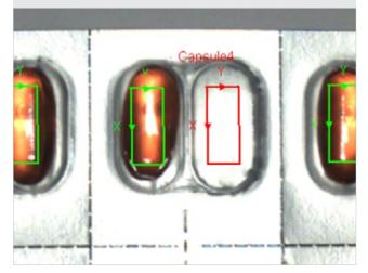
Brightness, contrast, pattern, pixel count, edge, and circle tools determine the presence or absence of a part.
