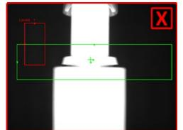
A lotion bottle is checked to confirm that the pump dispenser is in the locked position before the bottle is packed into a carton.
