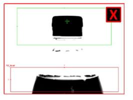
In-Sight vision sensors allow you to perform multiple inspections with each image. In this example, a bottle passes in front of the sensor, and both fill level and cap assembly are validated before the product is packaged.
