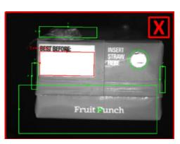
Inspections on a juice box verify that the date/lot code has been printed, confirm the safety seal is intact, check for the presence of a straw, and confirm that the flaps are fully secured.
