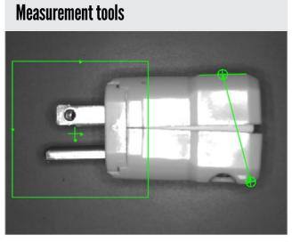
Distance, angle, and circle diameter measurements verify a part's features are the correct size and in the correct position and orientation.
