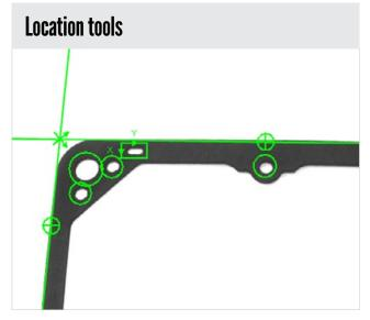
Pattern, edge, and circle tools locate (or fixture) the part so other vision tools can use this as a reference to complete their inspections.
