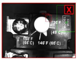
The dial on a thermostat is checked to confirm that it is in the correct position, which helps to ensure proper installation.
