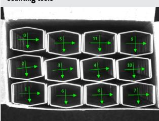
Counting patterns and edge features confirm the correct number of items are present on a conveyer or in a package.
