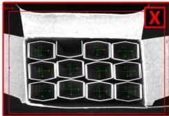
A pattern counting tool is used in this example to inspect the carton and to verify that the correct number of staple strips have been added.
