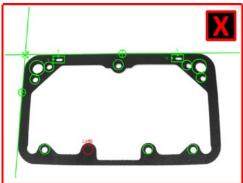
A fuel bowel gasket is inspected to verify that all 13 through holes have been punched out. A missing hole will cause the part to fail.
