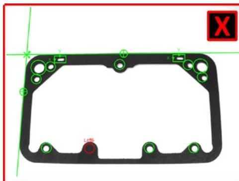
A fuel bowl gasket is inspected to verify that all 13 through holes have been punched out. A missing hole will cause the part to fail.
