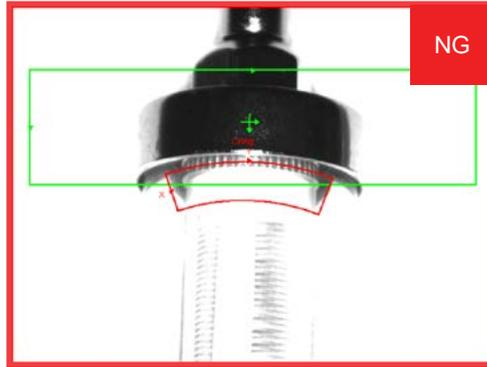
A fuel filter assembly is checked for the presence of an O-ring installed in the proper location before final packaging.
