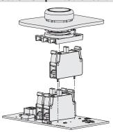
Versions with panel mounting of the EROUND series contact blocks with solder pin are available. If there is no wiring but a printed circuit, these contact blocks can be directly welded on the latter.
