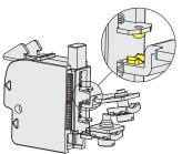
"V-shape" self-cleaning contacts with quadruple support point. This type of shape, thanks to the presence of the double support point, makes it possible to drastically reduce the probability of contact commutation failure. In addition to this, it improves considerably the reliability in the presence of dust.
