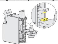
"V-shape" self-cleaning contacts with quadruple support point. This type of shape, thanks to the presence of the double support point, makes it possible to drastically reduce the probability of contact commutation failure. In addition to this, it improves considerably the reliability in the presence of dust.
