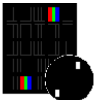
Cluster pixel defect type 1 Pixels in a cluster area constantly lit
