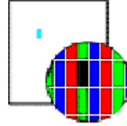
Pixel defect type 3b Sub-pixel/dot (red, blue, green) constantly dark
