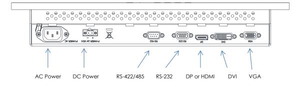
19":  ${}^{\oplus}_{\circ}{}^{\ominus}_{\circ}{}^{\ominus}_{\circ}{}^{\ominus}$ +°+°+° 00000 ဓိ္ဓ 6 1 Ā 6 0 0 è @.....)@ 1 DP or HDMI DVI AC Power DC Power RS-422/485 VGA RS-232
