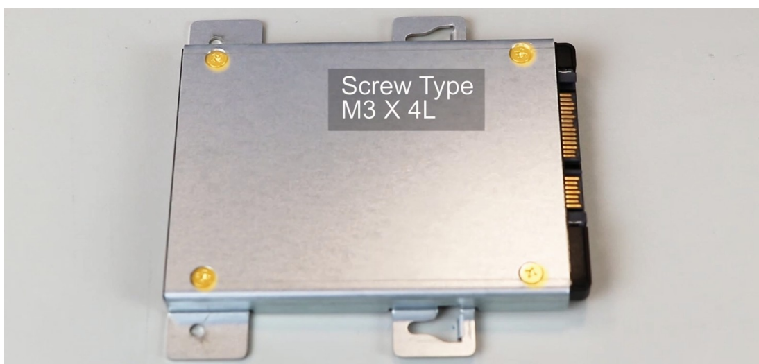
Figure 2.2 Install SSD - 2
