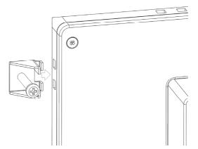
3. Secure the clamp to the panel using the included screws.
