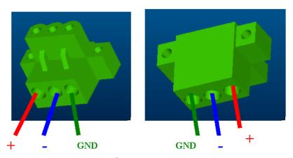
Figure 2.3 Power Connector and Power Lines
