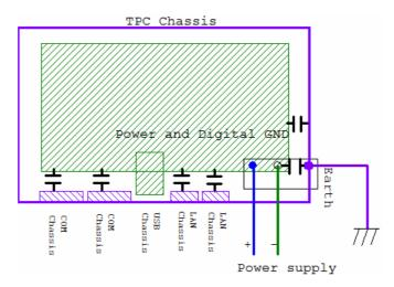
The TPC is and industrial grade product, designed to prevent external interference and the possibility of electric shock. To complete the isolation design, we need to consider the following:
