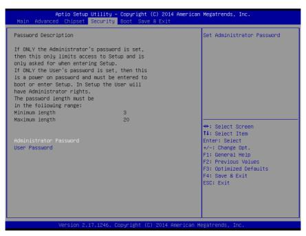
Select Security Setup from the Setup main BIOS setup menu. All Security Setup options, such as password protection and virus protection are described in this section. To access the sub menu for the following items, select the item and press <Enter>:
