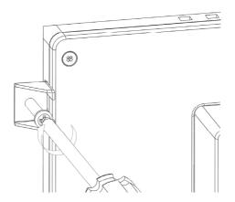
4. Smaller screws are included with the TPC-651T/TPC-651H, use these to avoid blocking CFast slot or I/O ports.
