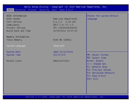
AMI's BIOS ROM has a built-in Setup program that allows users to modify the basic system configuration. This information is stored in flash ROM so it retains the Setup information when the power is turned off.
