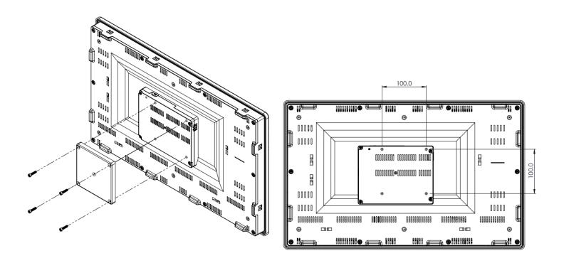
Follow the steps below to securely mount the USL-215-B05 using a VESA-compatible bracket:
