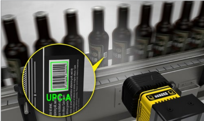
Barcode reading: Read codes on curved surfaces
