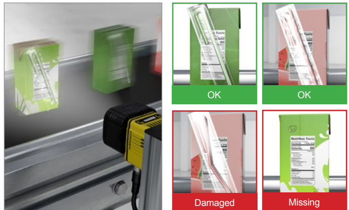
Food & beverage: Identify damaged or missing components
