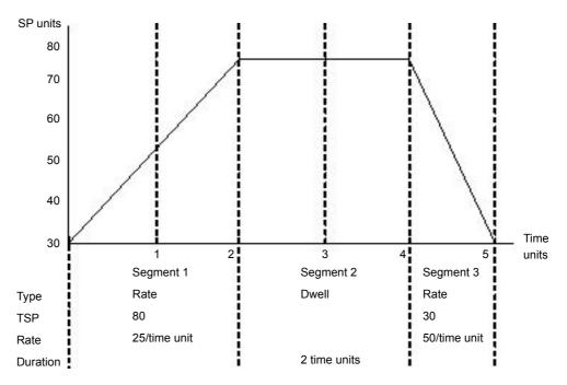
The example above shows a simple three segment program in which the Target Setpoint (TSP) increases at a controlled rate of 25/time unit to a value of 75. It then dwells at that setpoint for 2 time units before decreasing to 30 at a controlled rate of 50/time unit.
