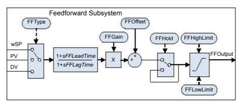
The Loop incorporates a feedforward controller in addition to the normal feedback (PID) controller; it is capable of static or dynamic feedforward compensation. Broadly, there are three common uses for feedforward in these instruments and are described in turn below.
