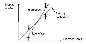
The procedure is exactly the same as shown in the previous section. For the minimum input set the 'CalValue' to the reading required on the controller as shown in the Low offset in the diagram above.
