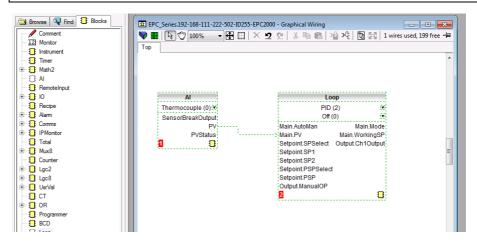
A list of function blocks is shown in the left hand side. Blocks are dragged and dropped from the list into the Graphical Wiring section on the right.
