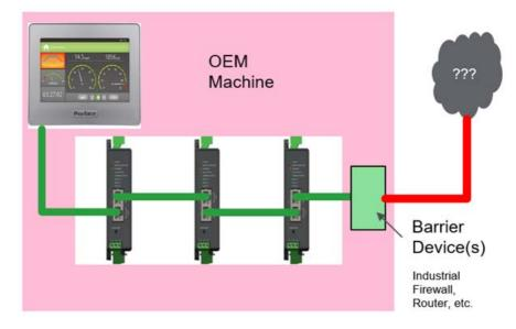
Additionally, it is recommended that the EPC2000 Programmable Controller 'preferred master' parameters are configured with the IP address of the HMI panel which will ensure that the HMI is able to connect to the EPC2000 Programmable Controller even if the other TCP sessions are currently active.
