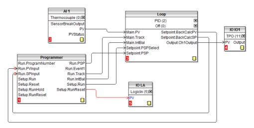
Soft wiring is carried out using iTools and is described in section "Graphical Wiring" on page 79.
