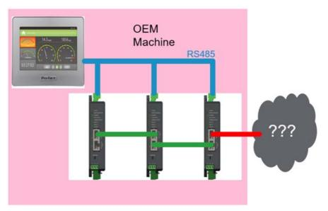
It should be noted that RS485 communications is given priority over Ethernet communications, however, RS485 is slow in comparison and therefore consideration should be given to the latency between the EPC2000 Programmable Controller and the HMI via RS485.
