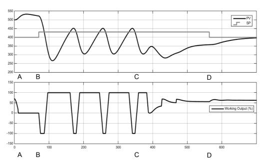
Autotune relies on the principle of cause and effect. It perturbs the process and then watches for what the effect will be. It is therefore essential that all external influences and disturbances are minimized as much as possible during an autotune.
