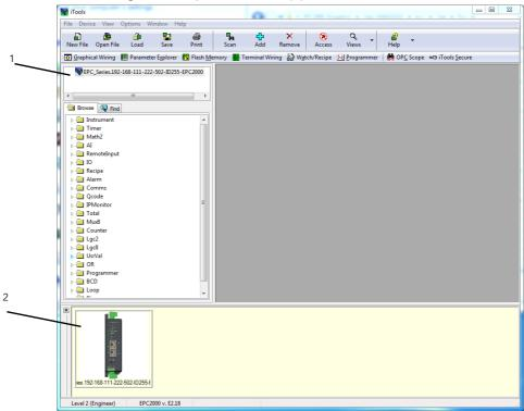
To maintain Cybersecurity best practise, it is recommended that AutoDiscovery is disabled when not required i.e.after Initial set up deactivate the AutoDiscovery function, for further details.see Auto Discovery parameter in "Comms.Serial.Network and Comms.Ethernet.Network" on page 127.
