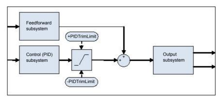
A symmetrical trim limit is provided around the PID component such that the influence of the feedback trim can be restricted.
