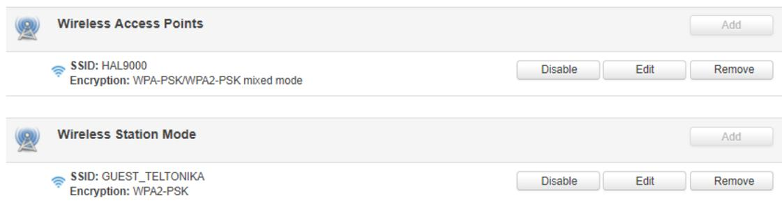
Above is the overview of the Wireless Configuration window. It displays active access points and stations. Here you can disable or enable your WiFi interfaces, remove unwanted access points or stations or enter a configuration window for each WiFi interface, where you can configure it more thoroughly.
