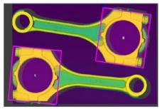
PatMax3D evolves the standard for finding parts. It ensures all vision tools are in the right location to accurately inspect the part on a 3D image.
