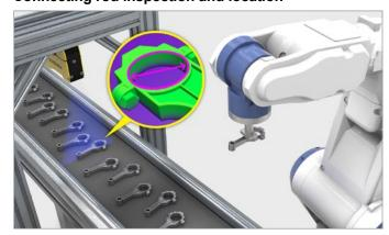
Locate the connecting rod on the belt using PatMax3D and measure the dimensions to ensure there are no part defects.
