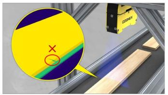
Inspect floor boards for orientation using the tongue. Check for defects along the surface including gouges, bowing, splits, and knotholes.
