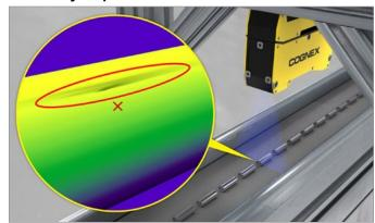
Detect dents, scratches, and other potential defects on the surface of an EV battery.
