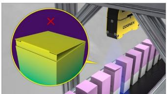
Verify the box is intact and sealed while inspecting for potential quality issues such as crushed corners, tears, or open flaps.
