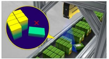
Inspect packages to determine correct number and proper orientation, including they have not fallen down. Also, check for defects in the packaging such as dents or tears.
