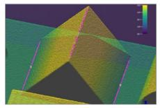
Edge3D uses the geometry of the part to reliably locate convex and concave edges on the 3D image.
