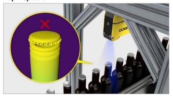
Ensure the bottle is properly sealed by checking the height and tilt angle of the bottle cap.
