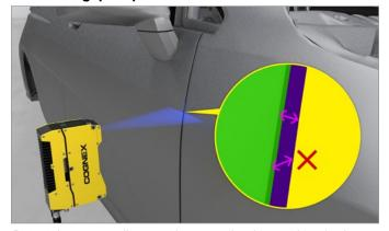
Detect the proper alignment between the door and car body, while ensuring the gap between the two is consistent.
