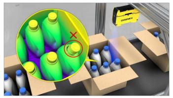
Verify the presence and position of the cap by checking the height and tilt to determine if it is screwed on correctly.
