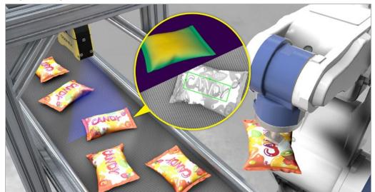
Locate a flexible food bag on the conveyor, identify its orientation using a combination of 2D and 3D tools, and inspect the volume to ensure there are no defects. Then, report the orientation to a robot down the line for packing.
