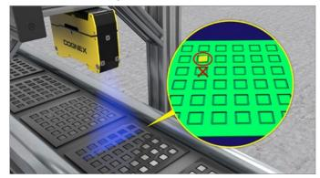
Determine if chips are correctly seated inside the carrier by measuring position and flatness.
