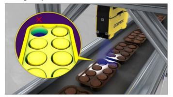
Determine the presence or absence of the part in packaging. Then, verify the volume of the package ensuring the correct amount.
