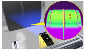
Locate the splice edge and verify the edge is straight on spliced rubber for tires.
