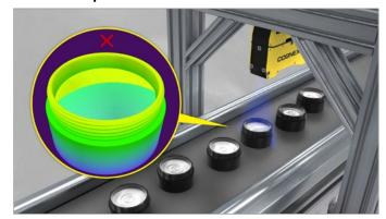
Inspect the height and volume of the contents to ensure that the correct amount of product is in each container.
