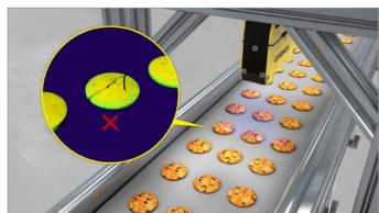
Verify the uniformity of cookies by measuring the length, width, and height. Plus, inspect for defects such as breaks or cracks in the cookies.
