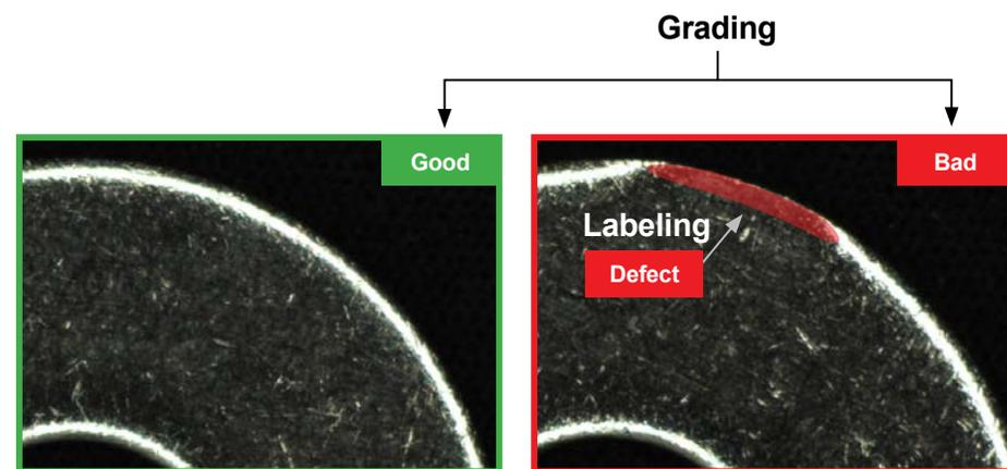
In this example, grading refers to the overall “good / bad” decision for each part, while “labeling” is the marking of specific defect pixels in the image.
