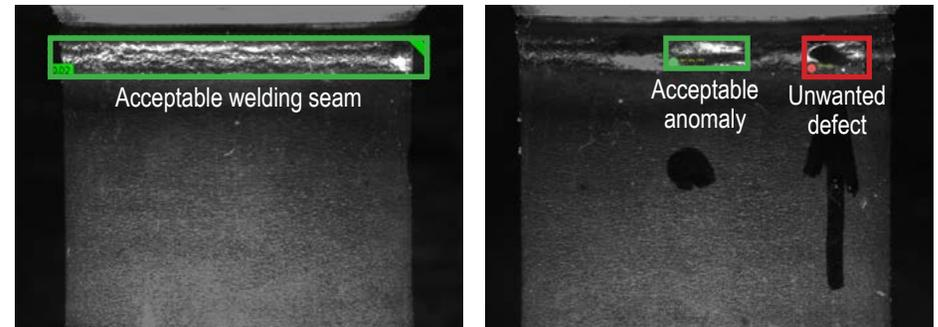
A piston’s welding seams are highly variable, making abnormalities difficult to distinguish. Certain welding anomalies, like missing or underfilled welds, cracks, or porosity, are unwanted. Other anomalies, like overlapping seams, are desirable and required for safety reasons. Dark image areas introduce additional complications. Given the many possible flaws and lighting challenges, deep learning-based analysis offers a simple and robust alternative to traditional machine vision inspection.
