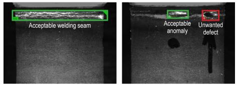
A piston's welding seams are highly variable, making abnormalities difficult to distinguish. Certain welding anomalies, like missing or underfilled welds, cracks, or porosity, are unwanted. Other anomalies, like overlapping seams, are desirable and required for safety reasons. Dark image areas introduce additional complications. Given the many possible flaws and lighting challenges, deep learning-based analysis offers a simple and robust alternative to traditional machine vision inspection.
