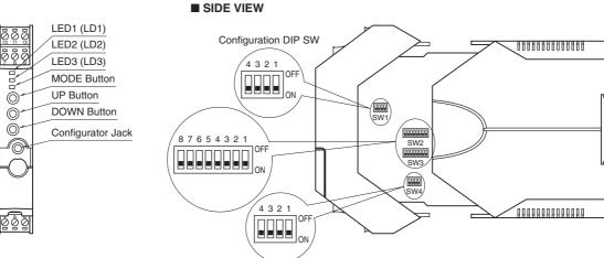
The DIP switch setting is required to select output types before setting a precise output range using the PC configurator software.
