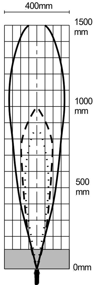
Beside the three typical cone shapes for the UPR-A sensors are shown (small, medium and large cone). Furthermore, the size of the detection beam is influenced by air temperature and humidity. The colder and dryer the air, the larger is the beam.
