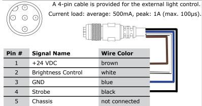
**NOTE** that this socket does not work if the external light is connected to one of the outputs on the I/O cable.
