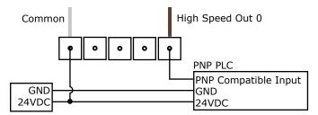
To connect the high-speed outputs to a relay, LED or similar load, connect the negative side of the load to the output and the positive side to  $\pm 24$ V. When the output switches on, the negative side of the load is pulled down to less than 3V, and 24 appears across the load. Use a protection diode for a large inductive load, with the anode connected to the output and the cathode connected to  $\pm 24$ V.
