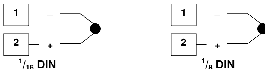
Figure 10. Thermocouple Input Connections
