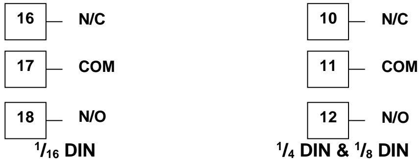
Figure 27. Option Slot 3 - Relay Module
