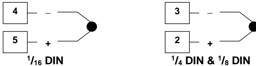
Figure 15. Thermocouple Input Connections
