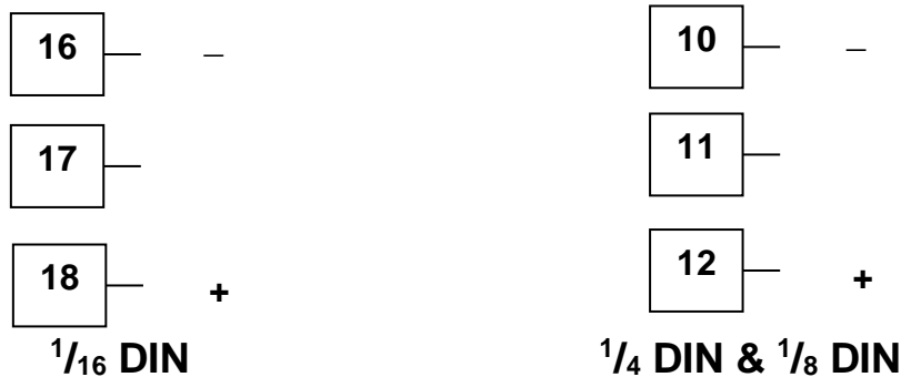
Figure 31. Option Slot 3 - Transmitter Power Supply Module
