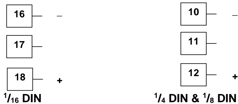
Figure 28. Option Slot 3 - SSR Driver Module
