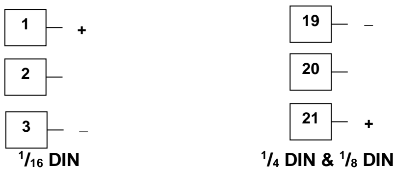
Figure 21. Option Slot 1 - Linear Voltage & mADC Module
