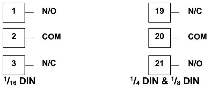
Figure 18. Option Slot 1 – Relay Module
