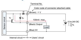
Symbols ... D : Reverse supply polarity protection diode Z<sub>D</sub>: Surge absorption zener diode Tr : PNP output transistor
