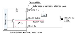
Symbols ... D : Reverse supply polarity protection diode Zo: Surge absorption zener diode Tr : NPN output transistor
