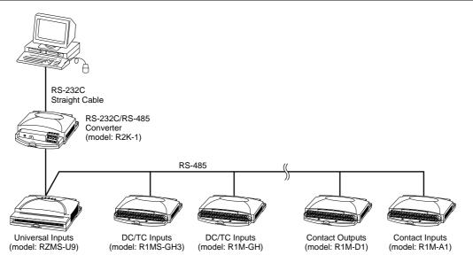
When the cable distance between the PC and the I/O modules is long, insert an RS-232C/RS-485 Converter for isolation.
