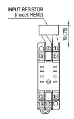
Input shunt resistor attached for current input.
