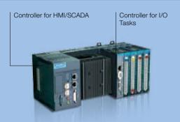
One controller focuses on I/O processing, while another controller can execute other tasks such as HMI/SCADA, database, recipe, image processing, etc. This architecture ensures system reliability since I/O processing won't be affected by other tasks.
