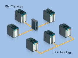
All APAX I/O modules are inserted on the backplane. Through the expansion port and Ethernet cable, different backplanes can be connected. This decentralized architecture retains high-speed data transfers, so the distributed I/O modules provide real-time performance. Almost any topology, such as line, tree or star, can be easily established. The hot swap capability is also available for remote expansion I/O modules.
