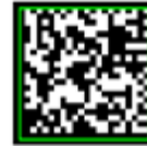
Quiet zone violation
