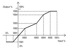
When the input is not defined in the user's table, two nearest value for each positive and negative are selected in written X. These two data are linearly interpolated and Y is obtained and output it.
