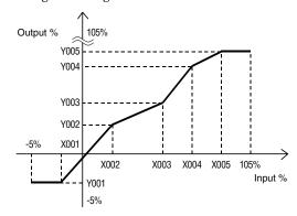
When the input is not defined in the user's table, two nearest value for each positive and negative are selected in written X. These two data are linearly interpolated and Y is obtained and output it.
