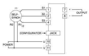
\*1. The output increases when the self-synch rotates clockwise. For changing the operation to counterclockwise and increase, set the ITEM 10 'Rotating direction' to CCW.
