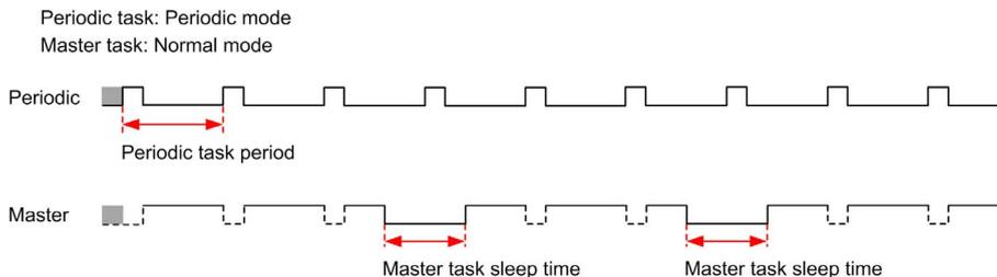
In freewheeling mode, the master task sleep time is at least 30% of the total cycle time with a minimum of 1 millisecond. This percentage may be higher depending on the user application (periodic task scan time, event task scan time, communication interaction, and so on).
