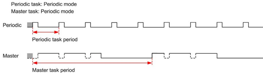
If the processor goes to the HALTED state when the master task is configured in freewheeling mode, verify whether the periodic task scan delay time is significant in comparison to the periodic task period. If so, try:
