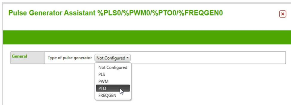
The **Pulse Generator Assistant %PTOx** enables you to configure the software parameters. A servo drive must be configured separately, refer to Configuring a Servo Drive with SoMove ([see page 20](#)). You must adapt the software parameters according to the parameters of your servo drive and motor.
