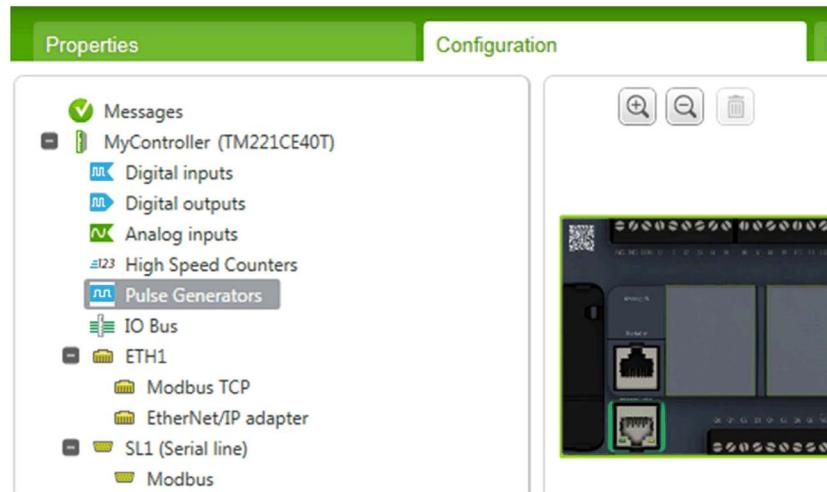
Except for the controller references with relay outputs, there are two **Pulse Generators** in the M221 Logic Controller that you can configure for various applications. You can configure both of them as PTOs and each output is called an axis in EcoStruxure Machine Expert - Basic.
