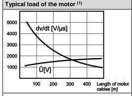
Load of the motor with overvoltage and slew rate when using conventional frequency inverters without integrated dv/dt filter chokes.
