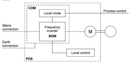
BDM: Base-Drive-Module Basic drive consisting of the power part and the control electronics
