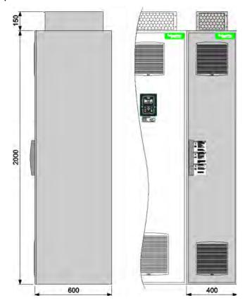
Interior View Braking Unit Option IP23 for Size 1c
