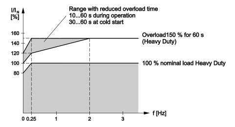
**NOTE:** If the frequency inverter is operated with output frequencies < 2 Hz the overload time at high overload up to 150 % is lower than 60 s. This restriction needs to be observed only for drives which continuously operate around 0 Hz and require overloads up to 150 %.
