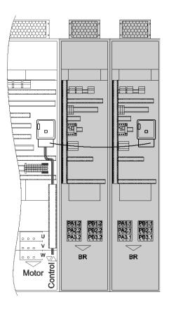
**NOTE:** At protection degree IP54 the enclosure height is increased by 200 mm.
