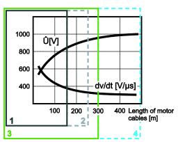
Reduced load of the motor by using Altivar Process Drive Systems with integrated dv/dt filter chokes 150 m (at higher types a "dv/dt filter choke" is already integrated).
