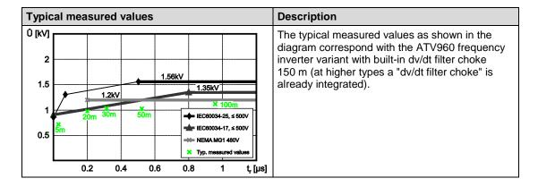
Motors according IEC 60034-25 as well as motors according NEMA MG1 are dimensioned for operation with frequency inverters and thus they are well qualified for drives with ATV960 frequency inverters.
