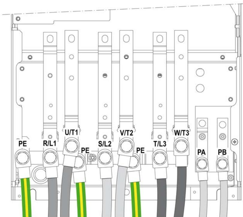
PA/+ and PB terminals are used to connect a braking resistor. Refer to the braking resistor instruction sheet [NHA87388](#) available on [www.schneider-electric.com](http://www.schneider-electric.com).
