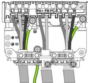
PA/+ and PB terminals are used to connect a braking resistor. Refer to the braking resistor instruction sheet [NHA87388](#) available on [www.schneider-electric.com](http://www.schneider-electric.com).
