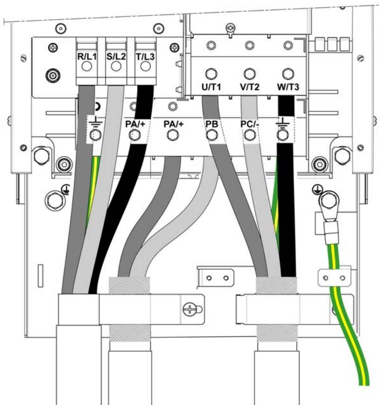
PA/+ and PB terminals are used to connect a braking resistor. Refer to the braking resistor instruction sheet [NHA87388](#) available on [www.schneider-electric.com](http://www.schneider-electric.com).
