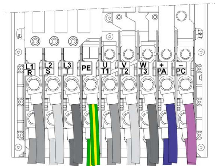
PA/+ and PC/- terminals are used to connect the braking unit. Refer to the braking unit instruction sheet [NVE16635](#) available on [www.schneider-electric.com](http://www.schneider-electric.com).
