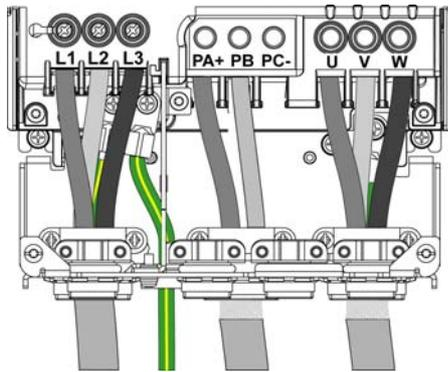
PA/+ and PB terminals are used to connect a braking resistor. Refer to the braking resistor instruction sheet [NHA87388](#) available on [www.schneider-electric.com](http://www.schneider-electric.com).
