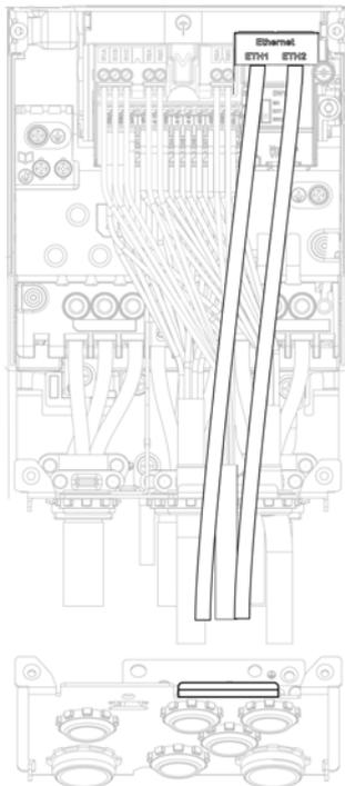
**NOTE:** Cabling plate shown is for frame size 2. Other cabling plates look slightly differs from this one.
