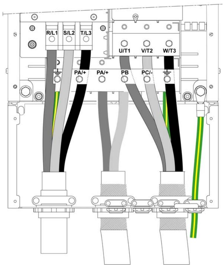
PA/+ and PB terminals are used to connect a braking resistor. Refer to the braking resistor instruction sheet [NHA87388](#) available on [www.schneider-electric.com](http://www.schneider-electric.com).
