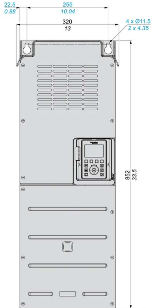
IP21 / UL Type1 Drives - Front, Rear and Side View
