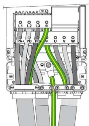
PA/+ and PB terminals are used to connect a braking resistor. Refer to the braking resistor instruction sheet [NHA87388](#) available on [www.schneider-electric.com](http://www.schneider-electric.com).
