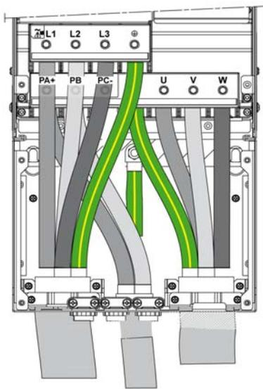
PA/+ and PB terminals are used to connect a braking resistor. Refer to the braking resistor instruction sheet [NHA87388](#) available on [www.schneider-electric.com](http://www.schneider-electric.com).
