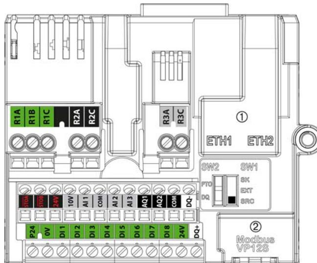
① Ethernet Modbus TCP, ② Serial Modbus
