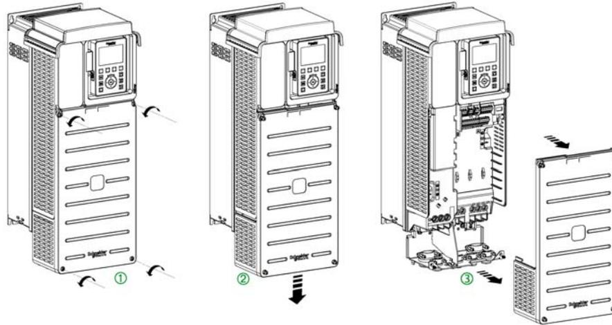
Apply the following instructions to access the terminals on **frame sizes 1 to 3** drives
