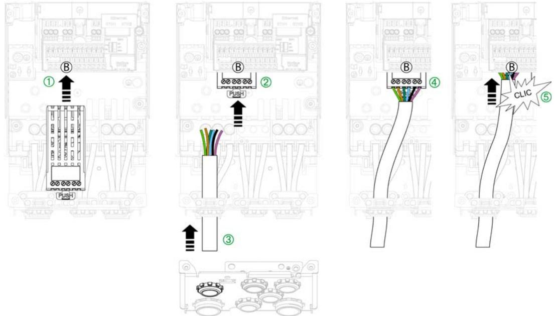
**NOTE:** Cabling plate shown is for frame size 2. Other cabling plates look slightly differs from this one.
