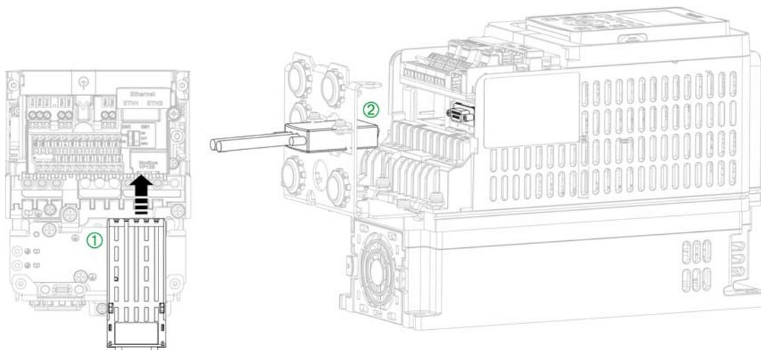
To help ensure correct wiring of the control part, apply the following instructions to install the PROFIBUS fieldbus module on Frame size 1 drives
