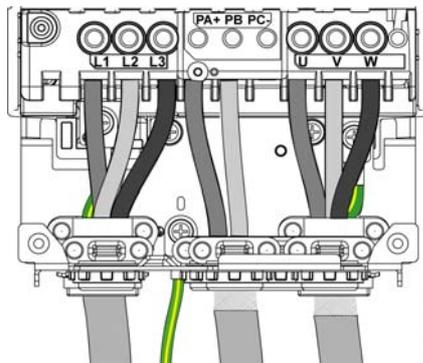
PA/+ and PB terminals are used to connect a braking resistor. Refer to the braking resistor instruction sheet [NHA87388](#) available on [www.schneider-electric.com](http://www.schneider-electric.com).
