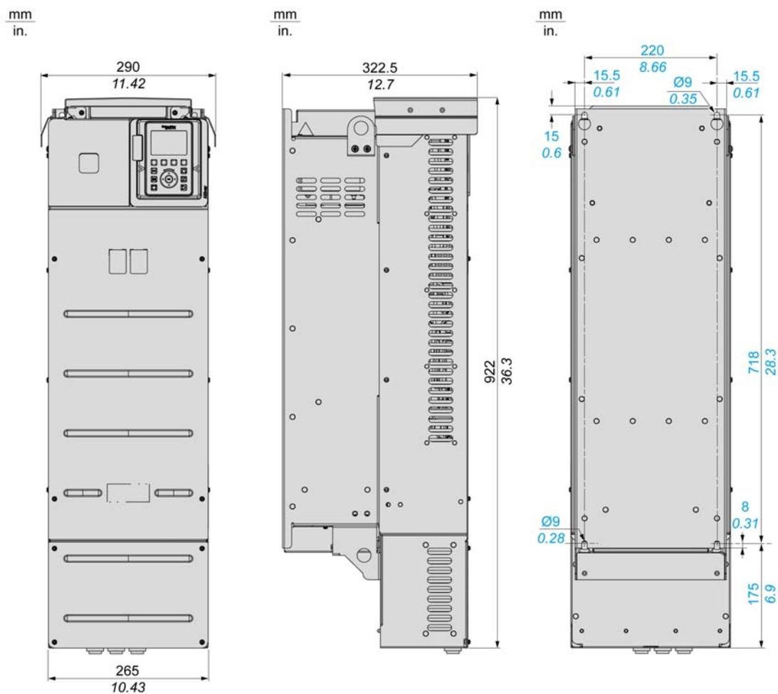
IP20 Drives, except on bottom side (IP00) - Front, Side And Rear View
