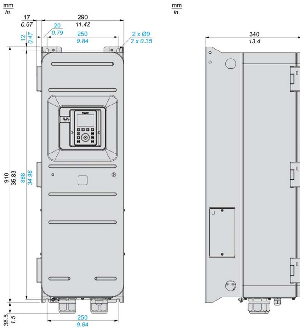
IP55 / UL Type 1 Drive With Load Switch - Front and Side view
