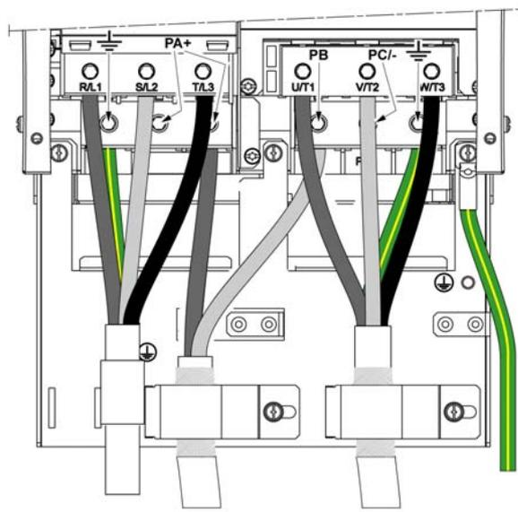
PA/+ and PB terminals are used to connect a braking resistor. Refer to the braking resistor instruction sheet [NHA87388](#) available on [www.schneider-electric.com](http://www.schneider-electric.com).
