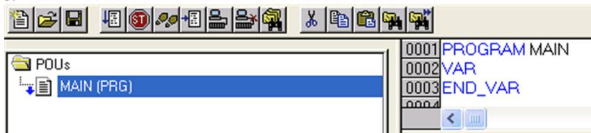
4. Check the compilation result without error; this action creates files in: *C:\TwinCAT\Plc\*, for example create *ATV\_PLC.tpy*
