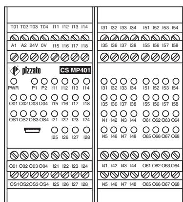
**Internal block diagram**
