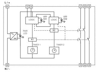
Y1-Y2: optional feedback inputs from any external contactors which are directly controlled by the module.
