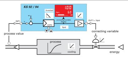
Fig.: 40 Normal 'cooling' - process
