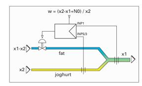
Fig.: 28 Ratio control = (x2 - x1 + N0) / x2
