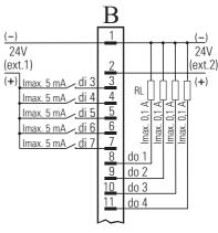
Digital input and outputs at two voltage sources (connector B)
