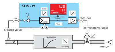
Fig.: 41 'Heating' process with inverting actuator
