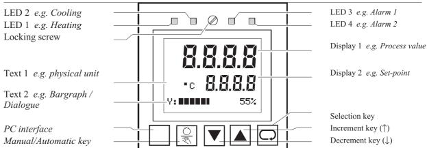
**Locking screw:** Locks the controller module in the housing.
