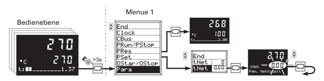
A preset time (parameter setting: Pmode = 1) can be entered in **hours** + **minutes** ( times < 99.59) or only in **hours** ( times > 99.59).
