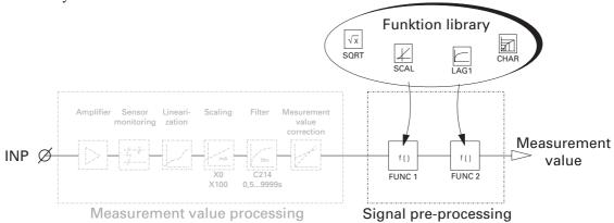
Each function can be used only once (either in Func1 or in Func2). The table gives a survey of inputs and usable functions.
