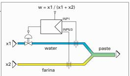
Fig.: 27 Ratio control = x1/(x1+x2)
