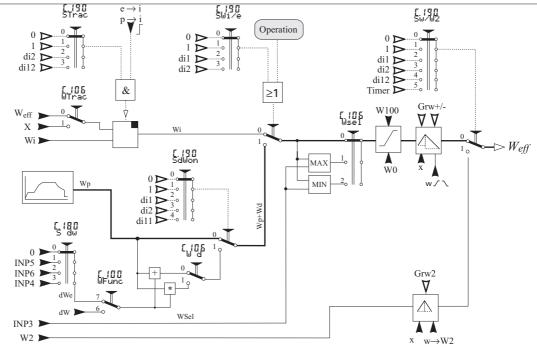
Fig.: 17 Programmer with ext. or int. offset [.100; WFunc = 6/]
