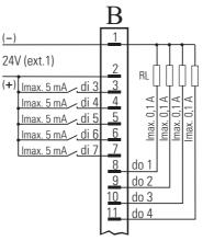
Digital inputs and outputs at one voltage source (connector B)
