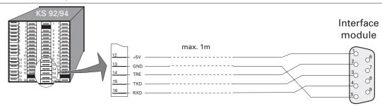
Fig.: 2 RS422-interface connection
