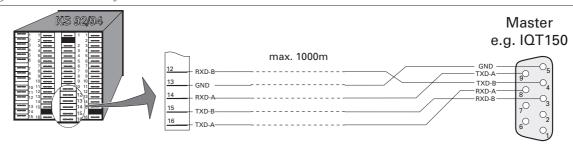
Fig.: 4 RS485-interface connection
