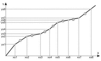
that there is a defined output value (ys) for each input value (xs). Beyond the defined intervals, the first or last segment is prolonged. Adjustable parameters: for each input - (x1,y1), (x2,y2)...(x8,y8)
