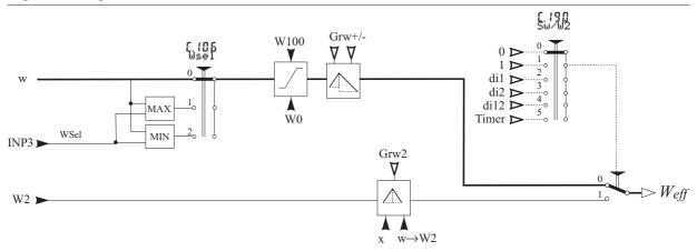
Fig.: 14 Setpoint / cascade control or programmer [. [00; WFunc = f or 2]
