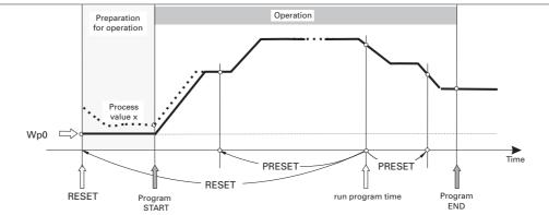
Fig.: 70 Profile with automatic reset at program end
