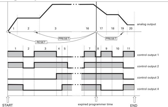
With respect to control signals and programmer visualization, the analog output is the master output. I.e. control commands act on the analog output (profile). Control outputs are forcibly tracked:
