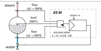
Fig.: 30 Block diagram for three-element control
