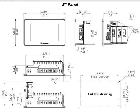
**NOTE** Allow space for modules to be snapped onto the back of the controller, if required by your application. Modules are available by separate order.
