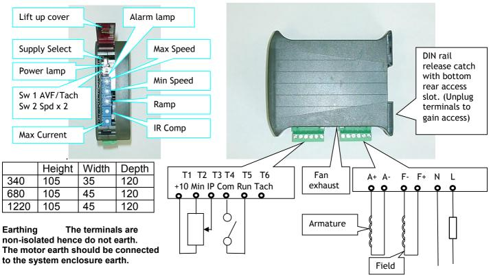
WARNING. This product is non-isolated hence all terminals are at dangerous line potential. Ensure connected items (e.g. speed pot, tach etc.) are not earthed and have sufficient dielectric strength to avoid breakdown.
