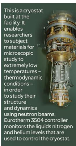
This is a cryostat built at the facility. It enables researchers to subject materials for microscopic study to extremely low temperatures - thermodynamic conditions - in order to study their structure and dynamics using neutron beams. Eurotherm 3504 controller monitors the liquids nitrogen and helium levels that are used to control the cryostat.
