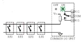
Fig. 20A – Relay de-energized, beacon ON lit.
