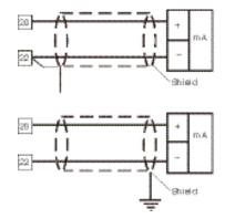
Fig. 6A – 6 mA INPUT WIRING
