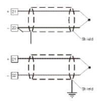
Fig. 4 – THERMOCOUPLE INPUT WIRING
