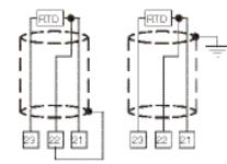
Fig. 5 – RTD INPUT WIRING
