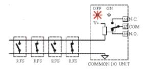
Fig. 20B – Relay energized, beacon OFF lit.
