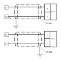
Fig. 6B – 60mV INPUT WIRING
