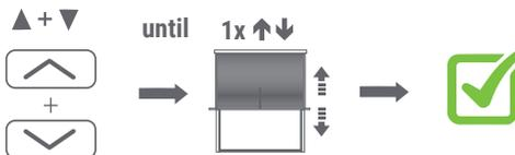
Press the UP and DOWN keys simultaneously until the motor moves up/down.
