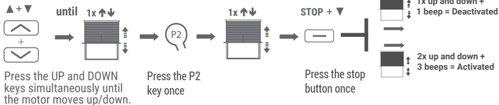
**i** Default is ON. The product will automatically check the upper limit every 50 times and adjust the top position. Please do not stop this process.
